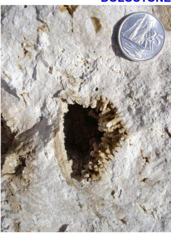
Formed of dolomite MgCa(CO<sub>3</sub>)<sub>2</sub>
